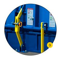
An integral safety stand works with the built-in maintenance strut to provide added safety during maintenance, servicing, and cleaning.\*
